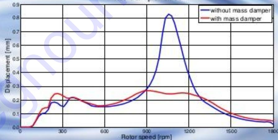
Frequency response measured on a vibrating machine
